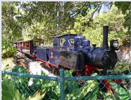
St. Nicholas Abbey Heritage Railway, a very short 2 ft 6 inches narrow-gauge railway. This locomotive, Tjepper no.5, was built in 1914 by Arnold Jung Lokomotivfabrik in Germany and was saved from a sugar plantation in Java in 2009. After being rebuilt in Tamworth, England, in 2018, it now operates from The Abbey to Cherry Tree Hill, just a very short distance, well under a mile.
